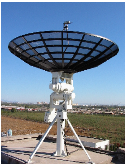
Example of 3.2 m X and L-band tracking antenna
